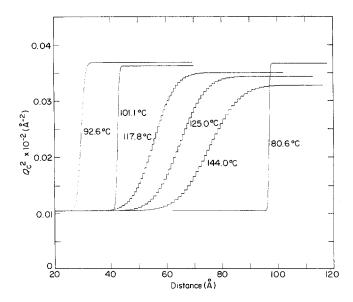
Figure 2 Density profiles of a deuterated PMMA/silicon interface at six different temperatures during a heating and subsequent cooling cycle. The origin of each profile on the x-axis, or the locations of the interface, was shifted by an arbitrary amount to illustrate the change in the profile shape. The ordinate is  $Q_{\rm c}^2$  and is linearly related to the local polymer density by a constant factor
