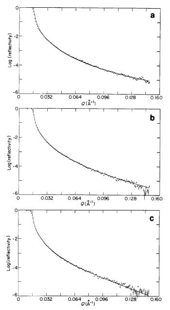
Figure 1 (a) Reflectivity curve from a deuterated PMMA/silicon interface at 92.6°C: (●) experimental points; (—) theoretical fit. (b) Same as (a) except the temperature was 117.8°C. (c) Same as (a) except the temperature was 144.0°C
