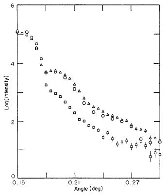
Figure 3 Results of a transverse scan from a deuterated PMMA/silicon interface at  $Q = 0.014 \text{ Å}^{-1}$ : ( $\bigcirc$ ) 92.6°C; ( $\triangle$ ) 101.1°C; ( $\square$ ) 117.8°C
